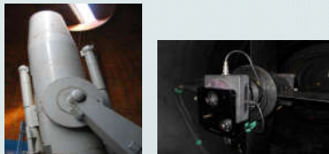
Fig. 1. 1m Schmidt telescope (left) and detector with filter wheels (right)
